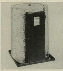
Hide-away water heater can be built into dead corner space in cabinets and save long pipe runs. Tank is extra-heavy guage galvanized steel, tested to over 300 psi. Extra thick insulation will keep water hot three days. Calrod units come in various wattages for 236-v systems. Heaters fit in 24" x 24" space, 26¾" high for 30 gal unit, 54 7/16" for 40 gal. Ten-year protection plan.
