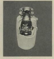
Sound-proofed disposer is enclosed in ½" of fiberglass and a polystyrene shell. It is suspended from the sink by a thick rubber cushion. Other rubber cushions separate the disposer and drain, form a seal across the waste feed hole. All moving parts are balanced to cut vibration. Imperial model has ⅓-hp motor, retails at \$129.95; Super is ¼-hp, \$99.95.
