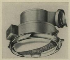
Extra quiet vent fans have 4¾" diameter squirrel-cage blowers and four-pole motors. This blower is used in three Ventrola ceiling models: 408, which is a ventilator only; 410, a ventilator plus light (above); 418, a ventilator-light-heater. It is also used in Model 806, a thin-wall unit for use in a shallow ceiling or a 4" stud wall.
