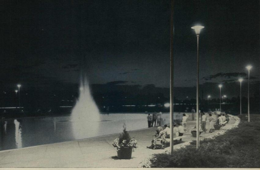
L-M'S PTLs were used to light this enchanting scene at the Ann Morrison Memorial Park in Boise, Idaho. Eighteen equally spaced 300 watt incandescent PTL luminaires, mounted on 20-foot aluminum poles, provide soft, low-level lighting for the gardens and walks surrounding the pool.
