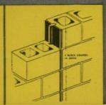
Rigid Backbone of Steel For Every Masonry Wall
