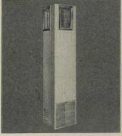
Compact furnace takes only 18"x18" of floor space, produces 50,000 Btuh of heat. It can be used in a closet or in a wall. Unit provides for up to four intake grilles at the bottom, hot air grilles at top. Unit is gas-fired, has ceramic-coated heat exchanger. Gravity upflow assures quiet operation. Furnace will continue to heat if electric power fails.
