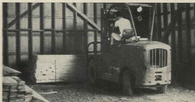
FORKLIFT TRUCK is one of two used almost constantly in the yard. They carry materials from trucks or boxcars on a rail spur to storage sheds, stack them, and load them on ten delivery trucks.
