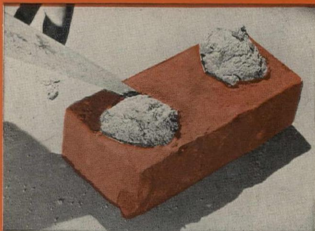
Place a dab of Brixment mortar and a dab of ordinary cement-and-lime mortar on a brick. Wait a minute, then feel each mortar.
