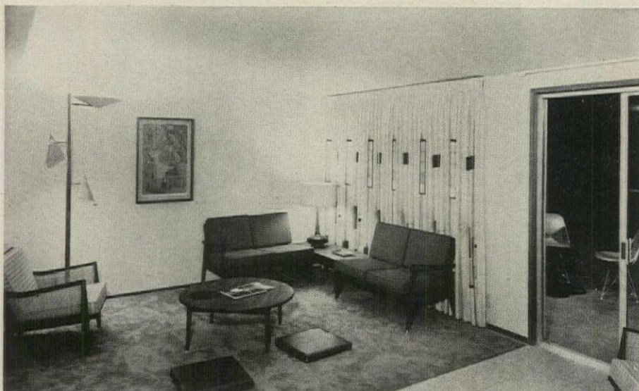
Living room has gently sloping ceiling that follows line of low-pitched roof and adds to open, airy feeling. Floor is terrazzo. Rear terrace, beyond sliding-glass door at right, is concrete.
