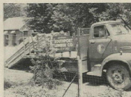
DELIVERIES are made on tight schedules by ten trucks. Lumber is sequence loaded to builders' requirement, strapped and then dumped at the site. Strapping prevents pilferage.
