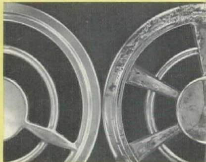
NuTone Anodized Grille (left) will not corrode like the ordinary chrome grille (on right).
