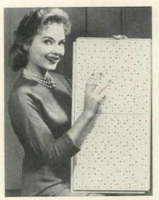
**Double-size tile** is 12"x24", center scored to give the look of two 12" tiles. Wood fiber tile is random drilled with three hole sizes. Calendered finish is smooth, washable, gives good light reflection without glare. Extended t&g edges allow hidden nailing or stapling.
