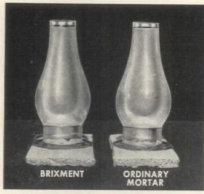
Prepare two slabs of mortar, one with Brixment and one with ordinary cement-and-lime mortar. After mortars have hardened, seal a lamp chimney to each of the mortar slabs, and fill with water.
