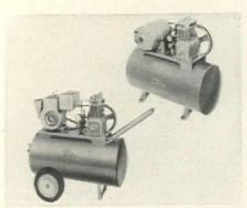
High-pressure air power is supplied by new Campbell-Hausfeld tank unit. Twocylinder compressor has a 2½" bore, 2" stroke, delivers over 4 cfm at 100 psi. Power is either 1-hp electric or 3-hp gasoline motor. 20-gal welded tank comes with 10" wheels or stationary mounts.
