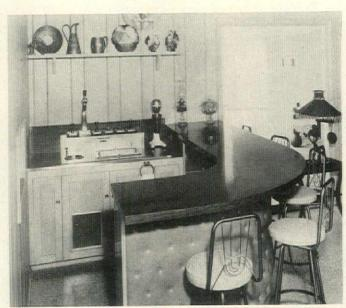
Home soda fountain and bar has three syrup (or liquor) pumps, two fruit compartments, carbonated water arm, running water dipper well, 5-gal ice cream storage. Coldwall refrigeration is powered by a 1/4-hp air-sealed compressor, keeps ice cream at 12F to 14F, cools complete unit. Carbonator makes sparkling water for 2¢ a gallon, 1/8¢ a drink. Fountain-bar is 321/2" wide, 237/8" deep. Service top is stainless steel. Price: \$665.
