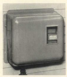
Outside meter box is made of weatherproof Kralastic, a rubber-resin material made by US Rubber. The meter box is big enough to take a variety of meter-regulator arrangements, can be suface mounted or recessed behind a front panel in an outside wall. Outside mounting allows meter to be read through a plexiglass window whether occupant is at home or not.
