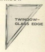
TWINDOW—GLASS EDGE. This type is just the thing for modern window-wall construction. Having exceptional insulating properties, it is constructed of two panes of ⅓\* PENNVERNON®—the quality window glass—with a ¾₁6\* air space between. TWINDOW—glass edge units are available in popular sizes for a variety of window styles.
