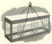
If hoisting is necessary, place sling so as to distribute load equally without distorting window in any way.
