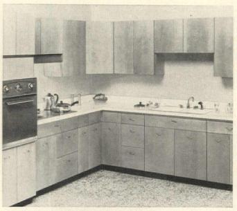
Beauty Queen kitchens' new line is called Fleetwood. Cabinet bodies are made of rust-resistant steel with baked enamel finishes. The fronts are solid-core, flush-front doors with white maple exteriors, birch interiors. Drawers made of one-piece die-drawn steel with wood fronts, roll on nylon wheels in interlocking rails. Hardware is anodized antique copper; cabinet closures are nickel alloy magnets. List price of 21" base cabinet: \$60.
