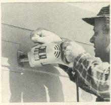
**Skil Recipro saw** works at two speeds to give faster cuts in metal, wood, plastics, fiberboard, etc. Model 700 serves as hacksaw, keyhole saw, or hand saw. Blade shoe moves to allow greater blade wear; off center blade allows cuts to corner. Unit delivers 3800 or 2500 strokes per minute. Stroke is 17/32". Price, complete with case and eight blades: \$99.50.
