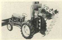
Everett trencher will attach to many makes of tractor, will dig a 24" trench 60" deep. Standard digging chain has eighteen 12" buckets. Frame has been strengthened at many points. New conveyor is positive acting, reversible, self cleaning, is curved to give higher spoil piles. Price: \$3300-\$4600.
