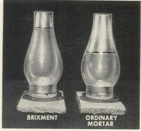
After 24 hours, note how much water has gone into and through the ordinary cement-and-lime mortar, and how little water has gone into or through the Brixment mortar.
