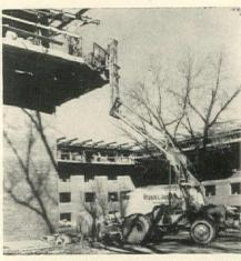
**Lull high-lift loader** will hoist 4000 lb 30' in the air for work with multi-story construction. The unit can be fitted with material buckets, forklifts (above), workman platform, concrete hopper or bucket, etc. Power is a 68-hp, 216 cu in. gasoline engine; speed is 25 mph in sixth gear. Price: \$7847-\$8691.
