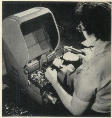
1. CALIBRATION In a dust-free room, where temperature is maintained at a constant 75°, operators calibrate every Pushmatic bi-metal assembly on a special optical viewer. Each bi-metal "latch" is adjusted to a dimensional accuracy of 1/1000 of an inch. Prior to this, the bi-metal had been heat-treated in an inert atmosphere to relieve stresses, "normalize" the metal.
