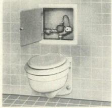
Residential flush-valve system makes tankless wall-hung closets practical for 3/4" piping. Air-loaded booster tank augments line supply to deliver two to six gallons per flush, refills in ten seconds. Flush valve has nylon diaphragm, may be electric or manually operated. Basic unit includes booster tank, flush valve, fittings, access panel, carrier, and wall-hung closet. List price: \$250. Haws-Kramer, San Francisco.
