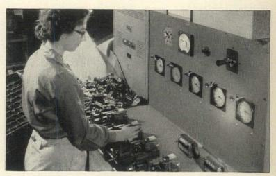
**3. CALIBRATION UNDER LOAD** Brought back to its "set" temperature, each breaker is checked at 200% of rated current, and again at the equivalent of 125% of rating. Check Boards are accurate to 1/10 of a second. Samples from each production run are also tested at 100% of rating.
