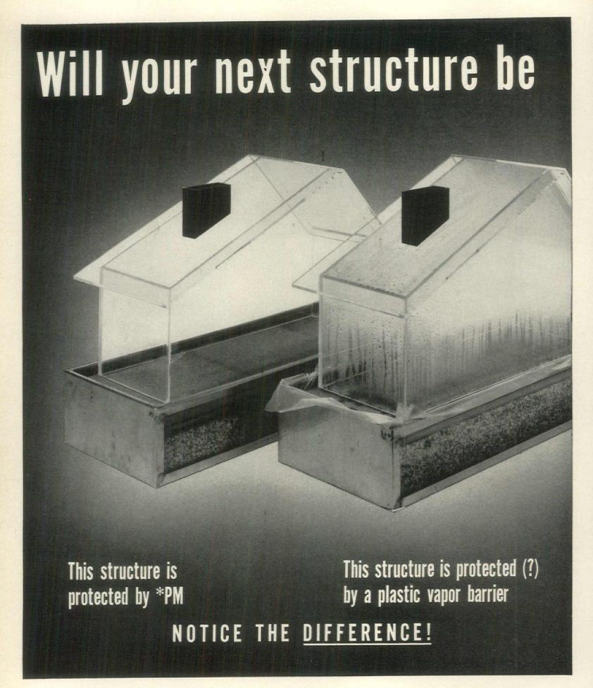
Pictured above is a display that has attracted widespread attention wherever it has been exhibited. Both houses, concrete slabs and tanks are identically constructed. The tanks are filled with sand, to represent soil, and water is added. On top of the soil is placed a vapor seal . "PM" under the house on the left and a plastic film under the house on the right. Heat is applied to the tank to accen-
