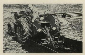
Auburn trencher is designed to work with Massey-Ferguson tractors. Variable hydraulic drive adjusts tractor speed to ground conditions. Unit will take trenching chains 6", 8", 10", 12", or 14" wide and booms up to 6' long. Hydraulic boom operates in 190° arc to control depth or backfilling under sidewalks, streets, etc. Auger-type conveyor spills dirt equally to each side. Special Pent-A-Bits are available for digging in rock, shale, or frozen ground.
