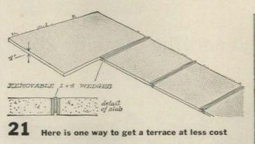
"I get concrete terraces and walks strong enough to withstand unstable soil by pouring separate blocks. When forms are stripped, we fill the joints with pea gravel or turf to match the yard." /END
