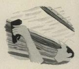
Fasten flange of blanket along inside ceiling joist with staples not more than 6 in. apart to form an air space  $\frac{3}{4}$  in. or more between gypsum board and vapor barrier.
