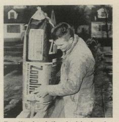
Zonolite insulation is claimed to improve U factor of an 8" cinderblock wall from .39 to .20 for only 10¢ a sq ft of wall area. Expanded vermiculite is waterrepellent treated, will not hold moisture, set up capillarity, or compact through settling. A 4-cu-ft bag will fill 16 three-core 8" blocks or 141/2 sq ft of wall. Bags are tabbed for easy pouring.
