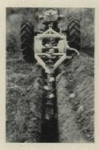
Deltec's Laster trencher will fit any wheeled tractor that has a live power take-off and ASAE three-point hitch. An "incher" device controls tractor speed. Adjustable high-carbon steel cutters will cut trenches 6" to 14" wide 4' deep at up to 500' per hour. Soil is carried to the right of cut by screw-type conveyor. A boom extension is available for deep trenching. Weight: about 700 lb.
