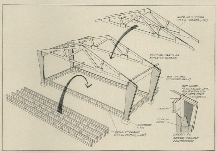
IN NEW FRAMING SYSTEM, built-up floor beams frame into two built-up main beams along sides of house which span from pier to pier.
