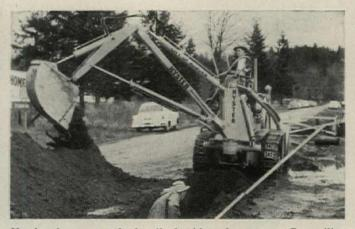
**Hyster** has a new hydraulic backhoe for use on Caterpillar D4 tractors or 955 Traxcavators. The unit will dig down 13', load to height of  $9'7\frac{1}{2}''$ . Full-power swing works through 240° arc. Buckets hold  $\frac{1}{2}$  cu yd, come in 13'', 21'', and 29'' widths. Back stay struts oscillate with tracks.
