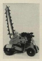
Arps M-A Trench-Devil is a medium-sized, self-propelled tool that will cut trenches 23/4", 31/2", 4", 6", or 8" wide, up to 54" deep, and up to 1200' per hour. Hydraulic drive lets you change speed or direction on the go. Hydraulic boom raises and lowers chain. Reversible rubber belt conveyor can dump dirt left or right of trench. The M-A can travel over the road on its own power at 23/4 mph.
