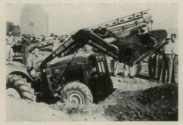
**Sherman Products'** new Napco four-wheel drive unit (left) adapts conventional tractors to work on difficult terrain. Power added to front wheels cuts digging into soft sand, side slipping on slick surfaces, backwheel spinning with front loads. Panther backhoe (right) has a compact 25-hp hydraulic system operating at 2000 psi, exerts digging force of
