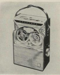
**Portable 2-speed recorder** holds an hour of on-the-job notes on a 3" reel of dual-track tape. Small (2%"x64%"x93%") unit is transistorized, weighs about  $6\frac{1}{2}$  lb. Mercury-cell penlight batteries run amplifier up to 300 hours, motor to 50 hours. Retail price, about \$200.
