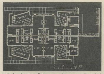
**PLAN** shows how two walls that separate four apartments form axis of building. Within apartments, bedrooms are isolated from living areas.
