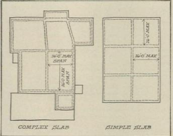
TYPICAL SLAB LAYOUTS show maximum spans between beams under slab. Ft Worth builders pour carport, planters, slab at one time./END
