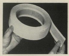
Metal-back joint tape is said to eliminate drywall joint lines, shrinkage lines, and ridging. Flexible steel backing is  $1\frac{1}{4}$ " wide .0075" thick, will bridge gaps to  $\frac{1}{2}$ " and more, will cover large overcut holes, openings at sills and jambs. The metal is centered on 2" paper tape, takes less cement, goes up faster than ordinary tape. Retail price, per 100', 4½ lb roll \$3.80. United Dry Wall Prods, Cleveland.
