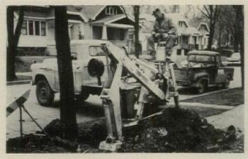
**Ottawa Model LX backhoe** fits many makes of trucks and tractors, digs to  $12\frac{1}{2}$  depths in any position on a 190° arc. Patented ejector bucket speeds work in muck, quick on-and-off mountings make for economical use of equipment. A front-end loader works off the same hydraulic system.
