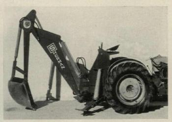
almost 20,000 lb. When swinging, drive elements are under tension and under positive control. In Ford installations the Panther has an electric-fan-cooled heat exchanger to keep unit working under extreme conditions.
