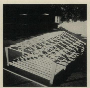
**SCALE MODEL** suggests that full-scale house could look like conventional house except for haunch shape of box columns. This shape is necessary to provide rigid (rather than simple "hinged") connection between columns and trusses. Sizes of dimension lumber and plywood in built-up beams and columns would depend upon size of house (ie, spans).
