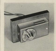
**Gas-heat modulator** is controlled by tiny thermistor which reacts immediately to small changes in temperature. Flame size is varied to maintain a steady ambient, eliminate off-and-on cycling. Usual thermostat acts as top-limit switch to cut off burner when atmospheric temperature rises above heating level. Blower operates continuously, prevents dead-air blankets. Price: \$82-\$94.
