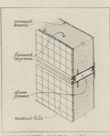
**MAUL MACOTTA PANELS** combine ceramic tiles with sandwiches of asbestos cement and insulation in an interlocking aluminum frame.
