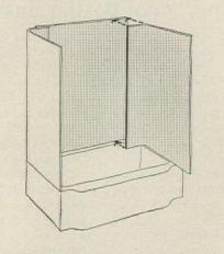
**THREE-PART ALCOVE** is made of a flat back sheet and two postformed end pieces.
