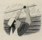
Staple flange to inside surface of next ceiling joist.
