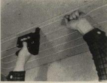
Radiant-heat tacker from Bostitch makes for fast, easy hanging of radiantheat cable or low-voltage wire. Special 7/16" long staples have shaped crowns. Driver is ground out to fit. Eastern price: \$14.25.
