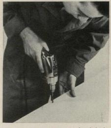
**ORDINARY TWIST DRILL** cuts clean holes in Glasweld as easily as it would in plywood.
