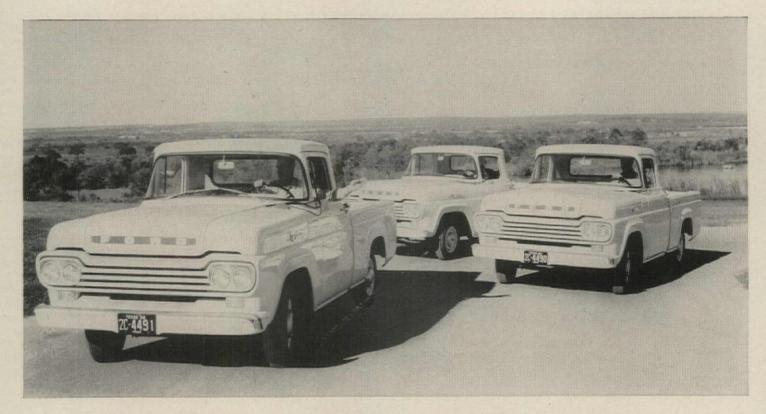
'59 Ford pickups running one of the Economy Showdown courses set up by the research engineers. Like all the new '59 pickups tested, these are regular stock models with a standard six-cylinder engine, 3-speed transmission and standard rear axle ratio.
