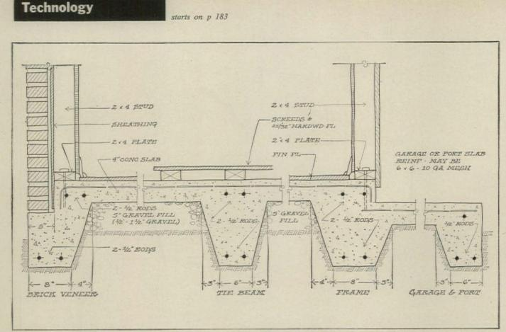
**CROSS-SECTION** of slab shows position of four  $\frac{1}{2}$ " rods in each perimeter and intermediate beam. The slab has a heavy waffle form,
