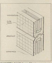
MARIETTA PANELS use Mosaic ceramics to face concrete-encased foamed plastic or foamed or fiber glass. Joint is mastic-sealed t&g.
