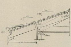
**CUTAWAY** shows how L-shaped plan works to give privacy to rear patio. Unusual feature of plan is the "family alcove" in the center of the house. Roof detail (directly above) shows how lookout is added to give change of pitch near eave.
