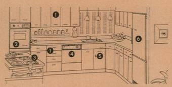
(1) "Select-A-Door"\* wall and base cabinets (2) Builtin gas or electric ovens (3) Built-in gas or electric cooking tops (4) Dishwashers (5) Disposers (6) Gas or electric refrigerator-freezers...plus automatic washers, gas or electric dryers, gas or electric washer-dryers, air conditioners, combination range-sink tops.
