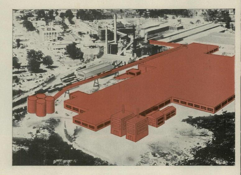
Shown (in color) are the new manufacturing additions to the Masonite plant at Laurel, Mississippi, which include new production lines, a new 26-boxcar loading dock, new research laboratories, new power plant, new office buildings and a revolutionary new raw-materials handling system.
