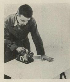
**SAWING** must be done with an abrasive wheel. Hard sheet would dull a steel blade.
