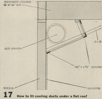
"When I can't put air-conditioning ducts into a dropped-ceiling hallway, or if ducts must run perpendicular to exposed ceiling joists, I put slanted furring around the duct. With some more thought, I'm sure the space above the furring could be used for storage or as a place to mount indirect lighting."
