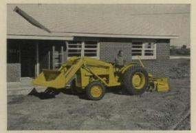
The Work Bull 202 with the Backhoe detached (you take it off or put it on in five minutes) and the M-F Scarifier-Scraper hooked up will scarify, level, back-fill, or scarify and level at the same time.
