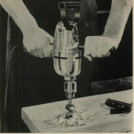
BLACK & DECKER'S U-21-A will drill 1/2" holes in steel, 34" in masonry, 1" in wood, or hole-saw 2". Geared chuck takes 1/2" shank.
