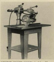
**NEWEST COMET MODEL** is 1-hp, 9" saw, uses two round arms. Double spindle takes tools at either end. Unit will cross cut 1"x12", rip to center of 50" panel. \$239. Comet Mfg Co, Los Angeles.
