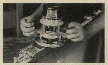
**STANLEY ROUTER** has new spotlight, chip blower, micrometer depth gauge, clamping lever, 3-grip handles to assure high precision, good visibility. %-hp model costs \$62.50; 11/4-hp model costs \$82.50. Stanley Electric Tools, New Britain, Conn.
