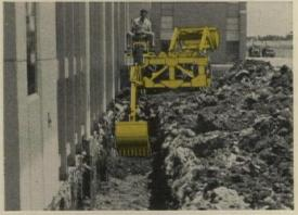
The Davis Backhoe is the only machine that will dig flush. 200° continuous operating arc lets you dig or dump to either side and never get cornered.
