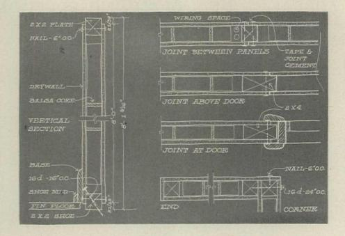
Detail of the "joint between panels" (near left, top) shows just how joint stud of one panel fits smoothly into the edge slot of the next panel. Note wiring chase left between edge of grid core and 2x2 joint stud. Panels are nailed together with 1/4" flat head, 11/4" long annular ringed nails driven 6" to 8" o.c. through the drywall into the joint stud of the adjacent panel.
