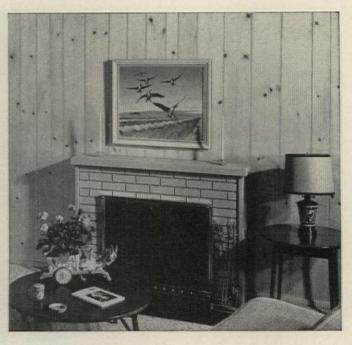
GRUVE-PLY: Idaho White Pine or Knotty Cedar plywood produced with surfaces carefully sliced like the most expensive imported woods. Looks like individual boards side by side. Goes up quickly, economically. Pre-grooved edges give uniform joints, eliminate need for mouldings.
