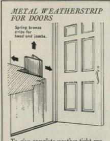
To give complete-weather-tight protection, doors as well as windows should be completely metal weatherstripped. Good metal weatherstripping gives buildings better protection against weather and saves more fuel per dollar of cost. Slide up the wood windows in this modern home . . . swing open the doors . . . and you'll find an important selling feature—modern metal weatherstripping.
