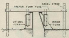
This new form is designed primarily for slab-on-grade foundations on housing projects. Also adaptable for any standard size, multiple re-use, low wall forming operation. It can be used for battered as well as straight walls. Standard dimensions of the form is 12 inches in height by 4, 6 or 8 feet in length. With proper care this form can be used hundreds of times.
