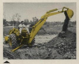
Ruggedly-built Case "320" backhoe, with exclusive hydraulic foot-controlled swing, digs hard clay with ease. Comfortable back-rest seat reverses for operating loader.
