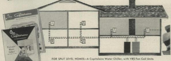
in every room (for both heating & cooling). For description of Water Chiller, get Form No. AC-937; VRS Fan Coil Units described in Form No. AC-859.
