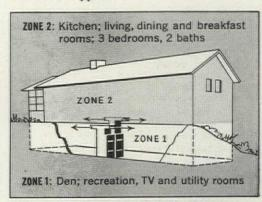
Zone 1—lower floor—uses 75,000 Btu input furnace; Zone 2—upper floor—uses 100,000 Btu input furnace.
