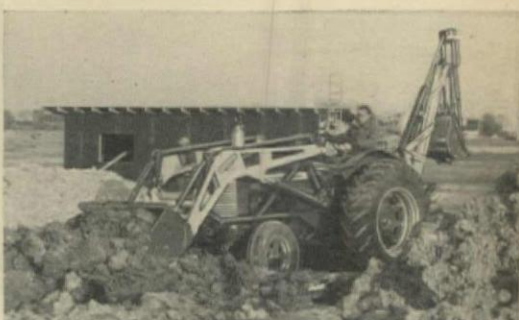
67 hp International 650 diesel gives you trenching capacity approaching that of small power shovels, with wheel tractor economy and mobility. Loads up to 2,500 lb, digs ditches to grade, as deep as 12 feet.
