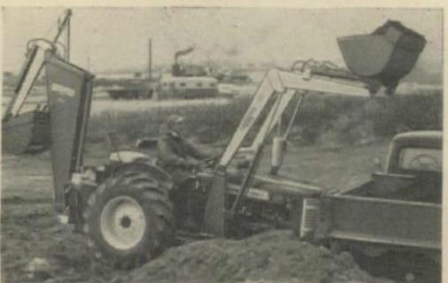
45 hp International 350, with gas, diesel, or LPG engine. Has the built-in brawn to handle ¾-ton with heavy-duty loader. Three models of heavy-duty backhoes match your job and your pocketbook for lowest cost.
