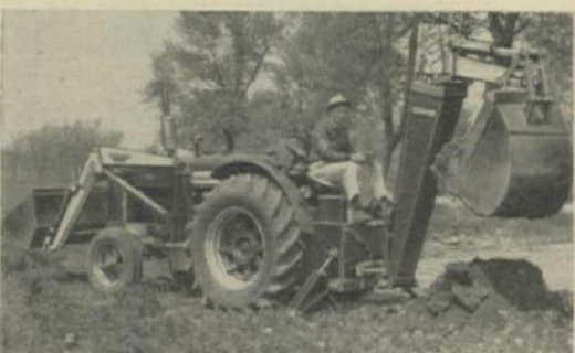
57 hp International 450. Over 6,600 pounds built-in operating weight. Loaders handle ¾-cu yd buckets, lift 2,000 pounds over 10 feet. Backhoes take bites up to 10 cu ft, dig 12 or 13½ feet deep.
