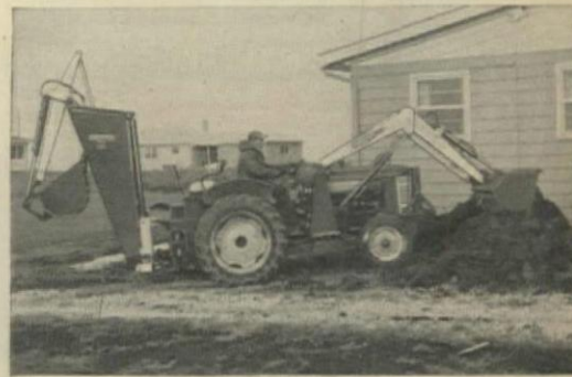
35 hp International 330. New and really rugged! Has the built-in "beef" to handle 1,000 pounds with front-end loader; step up yardage with choice of heavy-duty backhoes that maintain grades, digging 10 or 12-ft ditches.
