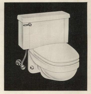
Since the unit has horizontal discharge, drainage collection can be above the floor, in the wall behind the unit. And since the floor underneath is clear (at its lowest point, the unit is 1½" off the floor), cleaning is easy and flooring can be installed without fitting around toilet base. Tank is standard size: 12" h., 21" w., 7" deep. Bowl is 15" h., projects 26". American-Standard Plumbing & Heating Div. New York City.
