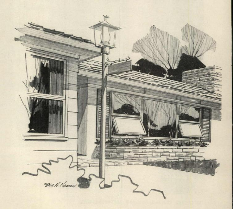
FOR THE ARCHITECT OR DESIGNER: new, slim joining mullion provides the advantage of attractive horizontal lines.
