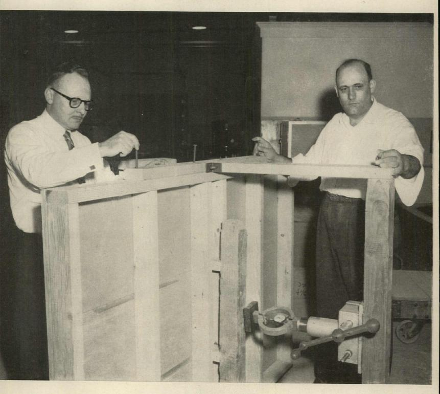
A series of tests on crack resistance of plaster corners was recently completed by Edwin L. Saxer, Professor and Chairman, Civil Engineering Department, Research Foundation, University of Toledo. Here you see the design of the test specimens, and the assembly of the testing equipment.
