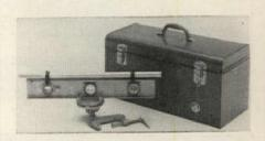
n. Magnelite sighting level comes complete with sighting tube (that has both a buckhorn open sight and a peep crosshair sight) mounted on the 18" protractor level. Turnplate head is calibrated and adjustable and the 4" graduated circle is movable so angles may be read from zero. It operates in 360° with graduations of 21/2°. \$29.95. You can get tripod of heavy gauge tubular aluminum as an accessory-it is interchangeable with Cclamp mounting. J. H. Scharf Mfg. Co., Omaha.
