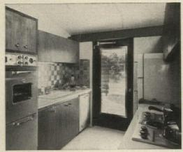
**BUILT-INS** (c) line sides of 8' x 12' kitchen. Cabinets are Samara plywood; wall tiles, stainless steel. Door leads to yard. Next to kitchen is utility room.
