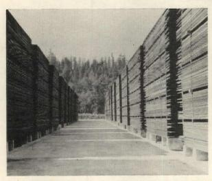
Each unitized stack is made up of lumber in classifications according to green weight, and remains in the yard until moisture content reaches a specified range.
