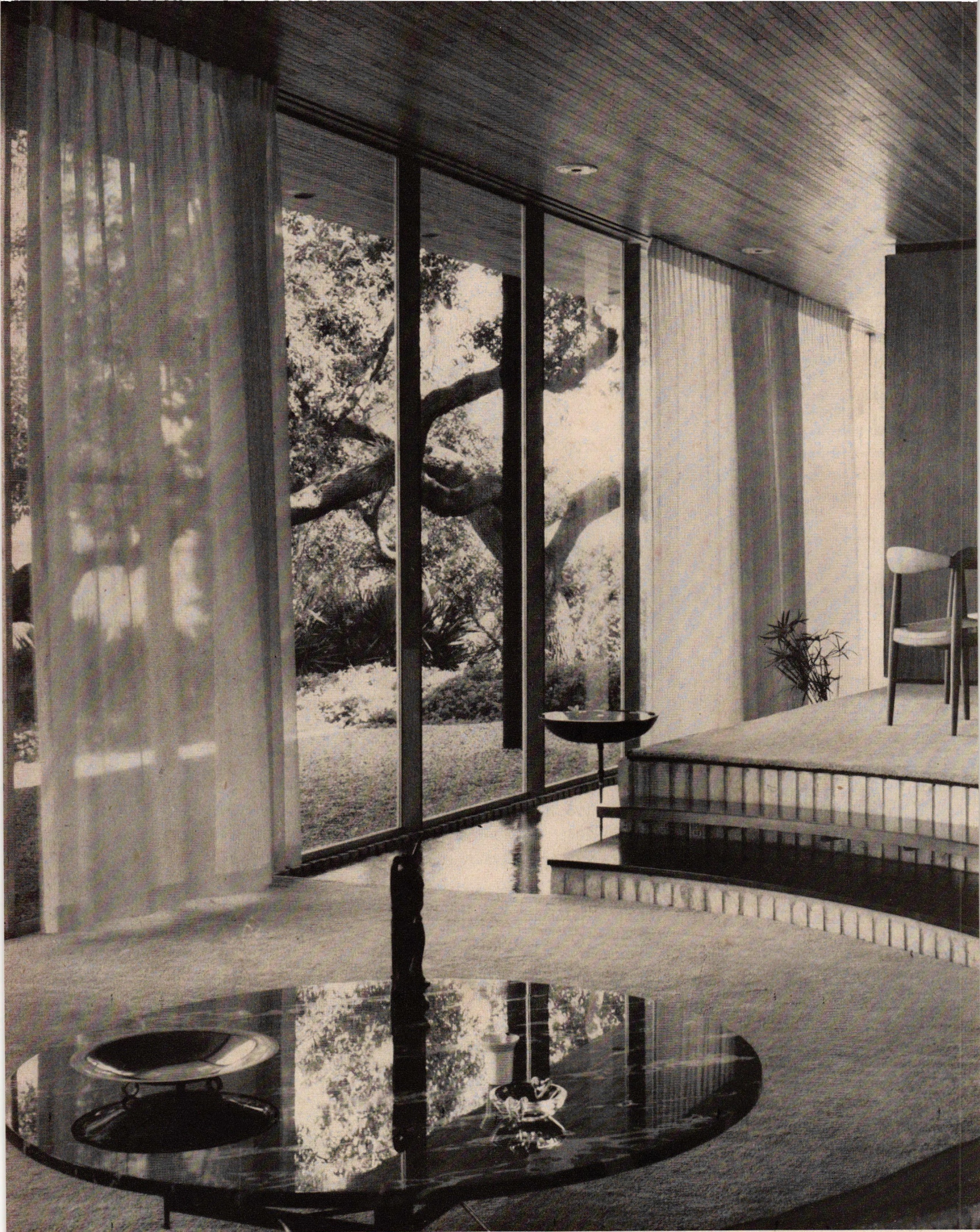
Mark Hampton's first award winner (see overleaf) takes advantage of easy-to-curve concrete masonry to set circles off against straight walls.
