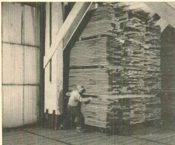
By the time lumber leaves the kiln, moisture has been pulled down to an average below equilibrium, and some surface moisture returned to stabilize equilibrium through each board.
