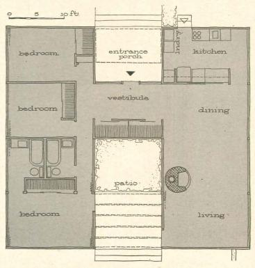
Plan shows simple, neat organization into two zones separated by 15' wide buffer. House would fit on a 60' lot.
