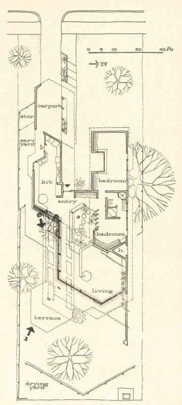
Plan of house (above) shows how, by combining long walls and angles and using fencing for privacy, the architect makes both house and lot seem spacious. When lot is long and narrow (diagrams below), turning house shortest distance limits space. Turning house long way increases possible length; angling walls continues view farther, makes house and lot seem larger.
