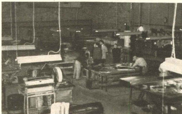
Fabricating ducts at Jack Segal's plant is an engineered operation for both air conditioning and hot air installations.
