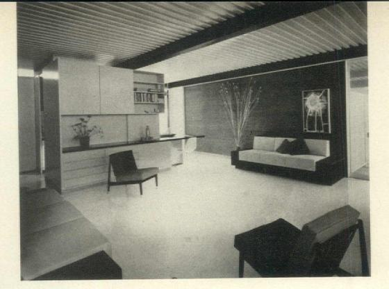
Because there are no interior structural supports, plan can be adjusted almost at will
