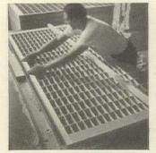
Stiles and rails securely fitted. Stiles are 11/6" instead of 11/8".
