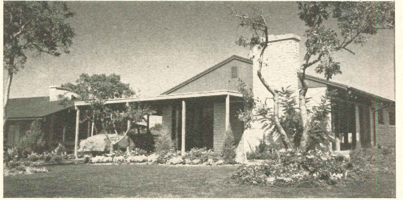
Model house placed narrow end to the street, gains width by addition of flat-roofed carport, strong horizontal line of covered walkway to entrance.
