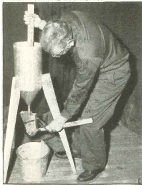
Mixing glue in this container is boon to production builders. Glue runs out bottom spigot into easily handled spreading machine.
