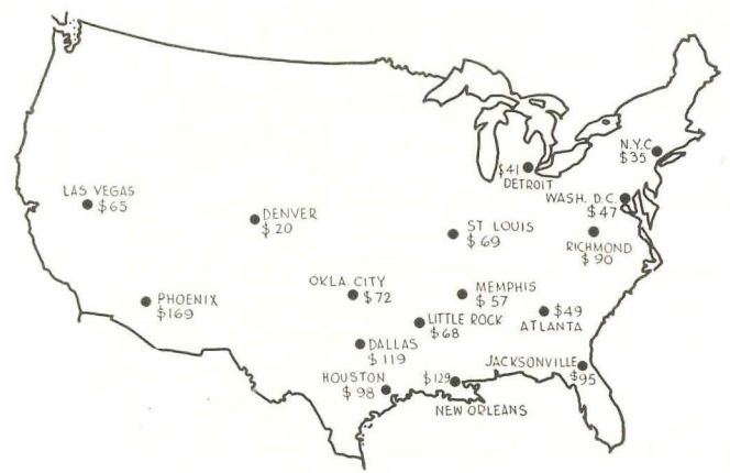
Map shows what cooling would have cost for same houses in random cities, based on $109 over-all average in Austin. Costs were estimated by H&H's technical staff, according to degree-days, and local electric rate for each city. Low cost in a hot city like Las Vegas is due to cheap electricity.
