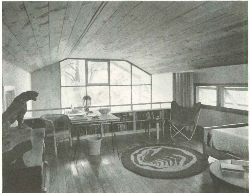
Study-balcony overlooks living area, gets plenty of light and handsome view through two-story glass wall. Dramatic living room was carved out of drab woodshed by imaginative device of ripping out part of old second floor. Long used by architects, this device is second only to glass walls as a means of adding spaciousness to an old house.
