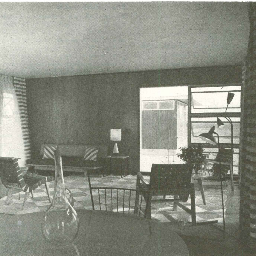
Cross ventilation is main objective of window placement, while 3" insulation batts in walls and roof ward off the heavy sun load. Living room is paneled in mahogany, rest of house is dry wall. Exterior planking is stained cypress.
