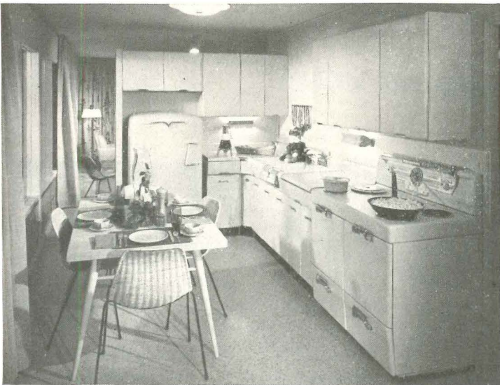
Work end of kitchen, seen from living end, is half open to more formal living room beyond. Freestanding partition ends 12" below ceiling, creates an air of spaciousness. Unbroken ceiling spans entire length of house. Note ventilating louvers under windows.
