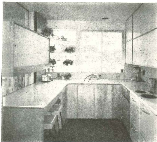
Open kitchen has efficient U-plan, plenty of continuous counter space, big windows up to top plate with view of front terrace and approach. Cabinet above pass-through has sliding hard board doors on both sides, hangs on black angle-iron posts. Stock folding partition, left, closes kitchen off.
