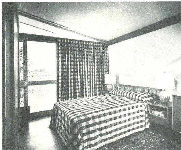
Frosted glass partition in top photo is optional item which not all builders use. Side walls are only 7' high, yet rooms appear normal height because of higher gable and sloping ceilings. Smooth-finished ceiling of plasterboard is in contrast with rough exposed beams used last year.
