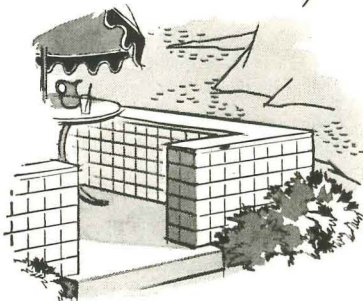
Here 8" x 8" units are stacked
