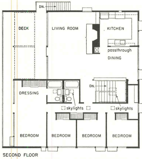
Upper floor locates main living spaces off ground for view and breeze. Back-to-back inside baths are skylighted.
