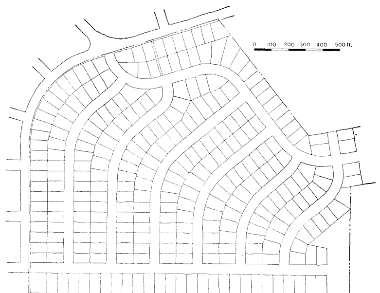
Lots for AEC's single houses average 62'-65' wide, would leave little space between 47' wide houses. Turning plan endwise makes house 14' narrower and alternating plans gives extra space between houses.
