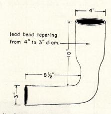
In earlier Levitt houses a lead bend below each toilet was made of 4" pipe. Now the lower portion is of 3" pipe, which saves about 4 lbs. of lead per fitting. The famous Jalonack plumbing tree will be used again. For photo see Feb. issue '51.
