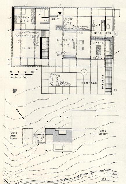
Here is another structurally in-line plan with post and beam framing. It shows what multipurpose space planning and cleverly designed built-ins can do: one end of the big living room serves as bar, dining room and guest sleeping quarters. It is easily maintained. Its design interest comes not from fussy "trim," but from structure and materials. It takes full advantage of its site and the view across a small lake.
