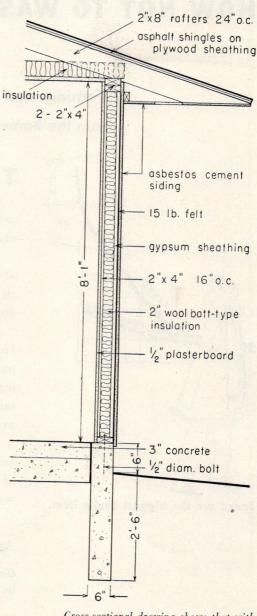
Cross-sectional drawing shows that with the exception of Levitt's asbestos cement exterior panel, construction is orthodox. Nailholes in asbestos panels are prepunched and nails are driven directly into studs, giving house more strength than if nails went into a sheathing.
