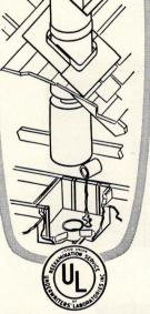
Van-Packer is tested and approved fire-safe by Underwriters' Labora-tories for all fuels. F.H.A. accepted. Has double-sealed, protecting joints —fire-clay tile liner and insulating vermiculite concrete wall equal in in-sulating value to 24" of brick or 70" of ordinary concrete.
