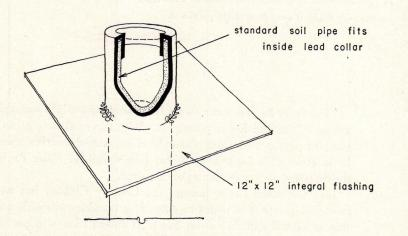
Levitt takes advantage of the shorter vent pipe projection sanctioned under the new national plumbing code to slip a flashing collar over the whole vent, thereby getting a more permanently waterproof job with almost no site labor cost at all. To save critical copper, the collar is made of lead.
