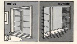
Durable aluminum alloy extrusions are the modern answer to the home-builders demand for the finest in window trim. These sills and stools, designed to take hard wear. eliminate maintenance, rust and rotting problems. This window trim stays bright and new-looking after years of service. Easy to install with regular tools, these Reynolds Aluminum window sills and stools fit right in with modern aluminum windows.
