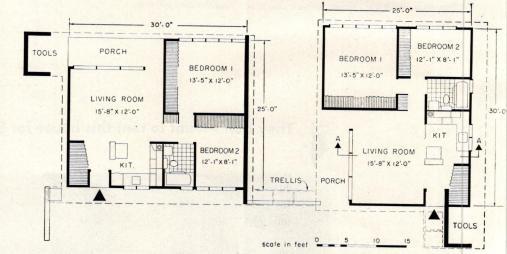
**THE BUDGETEER** has much in common with the two other new Levitt houses: Exterior wall panels are the same asbestos cement; slab, wall construction and interior painting are the same. But this is the Levitts' first flat roof. Kitchen has stainless steel sink, automatic washer, electric range, refrigerator. Bathroom is equipped like Levittowner. Each unit has 36 sq. ft. of outside storage.
