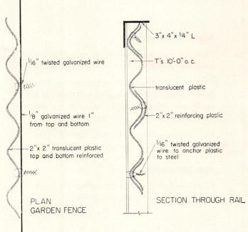
Because plastic material does not have to be drilled, detailing is simple.
