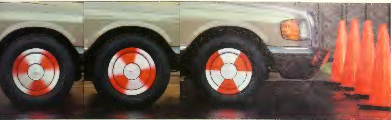
braking action as often as 10 separate times. Preventing wheel lockup—and keeping the car precisely steerable throughout.
