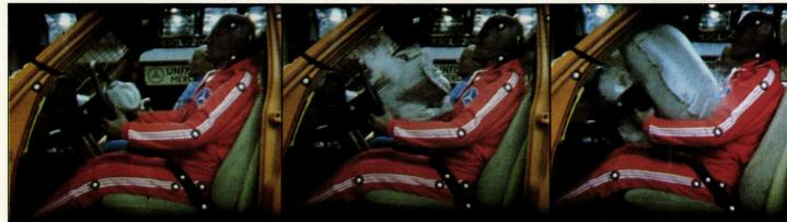
High-speed photography records a test deployment of the Mercedes-Benz Supplemental Restraint System. Within forty-fiv
