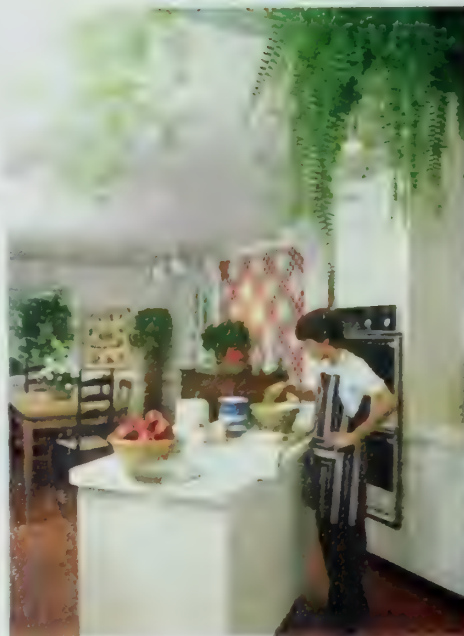
Above: Food consultant Freddi Greenberg at work, at home. The roll-around island is a stock cabinet with a counter added on top and casters added on the bottom. All cabinets are faced with laminate inside as well as out, to help prevent warping, simplify cleaning.
