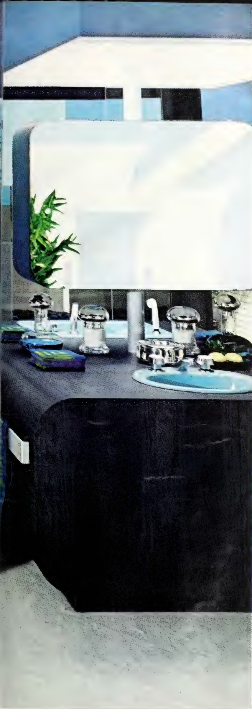
In wash-up make-up table: back-to-back basins, one round, one angular—the latter specially fitted with hand shower. Both are held by a plastic grid hung from ceiling.
