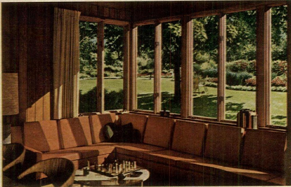
Cheerful windows with a "built-in" plus. They're TWINDOW insulating glass—two panes of glass with a layer of dry air sealed in between. TWINDOW keeps your home cooler in summer, warmer in winter. You get all the view and weather protection, too! For your free booklet about TWINDOW insulating glass, write to PPG at address given below.
