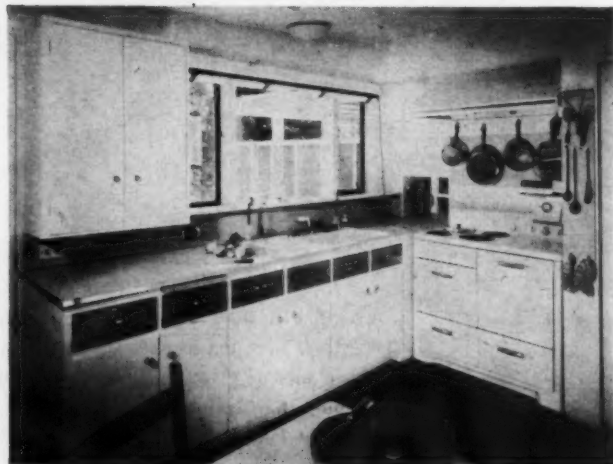
THE KITCHEN COUNTER beside the range is the same height as the top of the dining room buffet, forms a pass-through for dishes.
