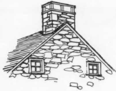
FIELDSTONE CHIMNEY has top which keeps out rain and down drafts.
