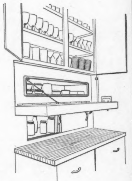
Over the bar counter is a cold cupboard for appetizers, etc., an ice-tray shelf, cabinet for glasses. The counter itself, like two others in the kitchen, has a top of heavy maple wood for chopping.
