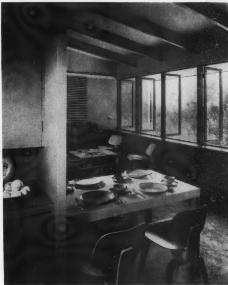
THE DINING-ROOM TABLE is in the living room but placed so it is right next door to passageway given over to linen, china, glass, silver. Kitchen is just beyond. View can be seen from the table through continuous bands of casement windows, under wide overhang which eliminates glare from the sun.
