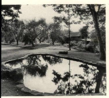
Ornamental as well as useful is the informally designed swimming pool. Simulating the contours of a natural pond, it was made by lining a bowl-shaped excavation with reenforced concrete. Stone edging comes from a river bottom.
