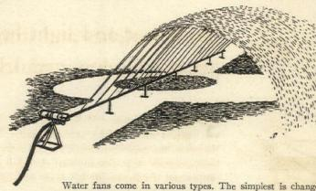
Water fans come in various types. The simplest is changed by hand. Others are swung mechanically from side to side. In this way a wide area is sprinkled with the least effort.
