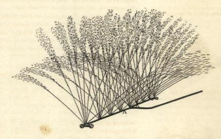
In this type of water sprinkler both farther spots reached by the fan are watered and also the immediate area alongside the perforated pipe. A strong force of water is required.
