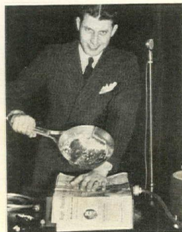
THIS cold stove will fry an egg but will not burn a newspaper. By electric induction the molecules of the frying pan are rapidly magnetized and demagnetized, bump together, generate high temperatures. General Motors
