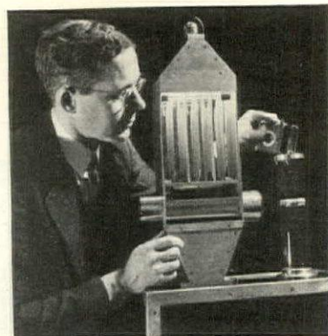
THIS "Precipitron" is designed for more efficient air cleaning. It first shoots a positive charge of electricity into the dust particles which, thus ionized, are drawn to a series of negative collector plates. Westinghouse
