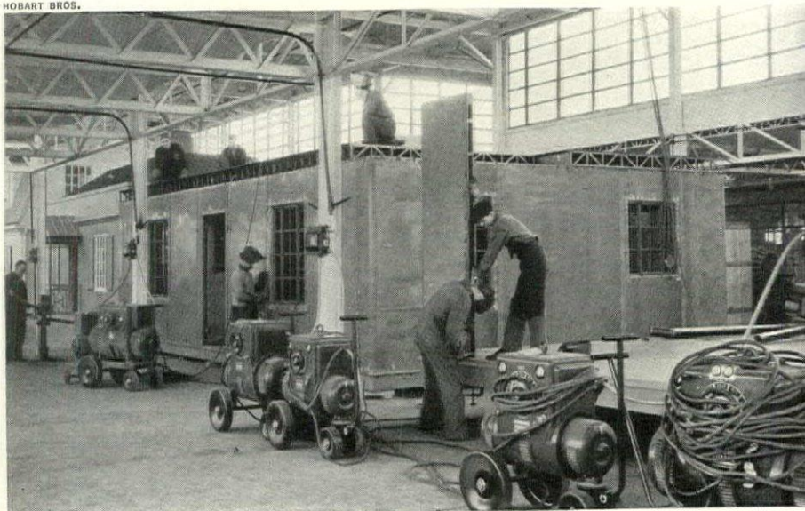
THIS WELDED METAL HOUSE IS BUILT ON AN ASSEMBLY LINE, LIKE AN AUTOMOBILE, THEN—
