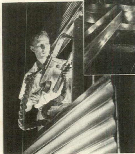
ABOVE RIGHT: The beginning of a modern railway coach. Strips of stainless steel are fed through a series of rollers, and then pressed into various shapes for structural members and exterior sheathing
