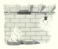
FIRE FINDER. An appliance so sensitive to sudden heat that it will instantly give warning of the smallest fire is now available. It is attached to the ceiling, or hidden from sight behind a grille in the ceiling and by its reaction to the presence of fire will attract attention to the hazard before it has had time to spread. When any sudden rise in room temperature approximates 20 degrees per minute the fire finder will sound an alarm.
