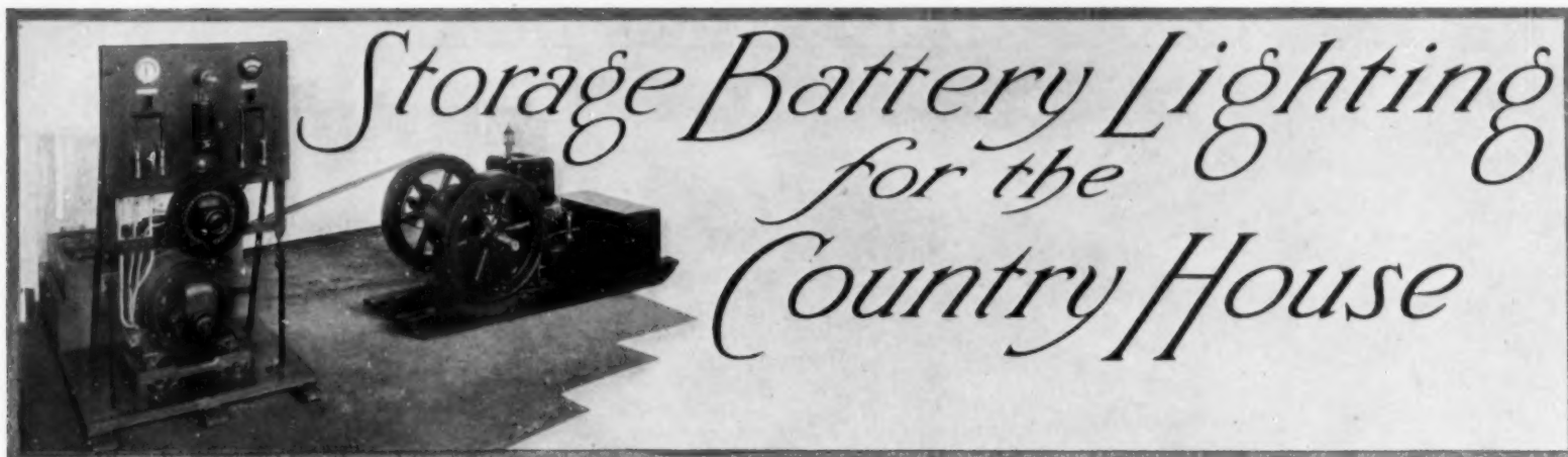
A low-voltage plant for a small house capable of supplying twenty-four 16-candle power bulbs, showing the simplicity of the complete plant
