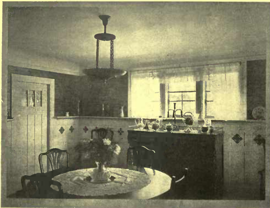
The glass bowl with a cluster of lights inside shows a faulty attempt at indirect lighting. A powerful reflector should be placed in the bowl throwing all the light on the ceiling. Small auxiliary lights beneath this would bring out the beauty of the glassware
