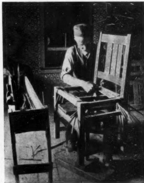
With the chair fastened upon a swivel post the weaver moistens his rushes and works around the frame
