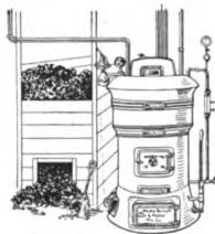
The low pressure steam boiler is very simple and safe in operation
