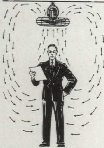
Above sketch shows air movement produced by the RECO.
