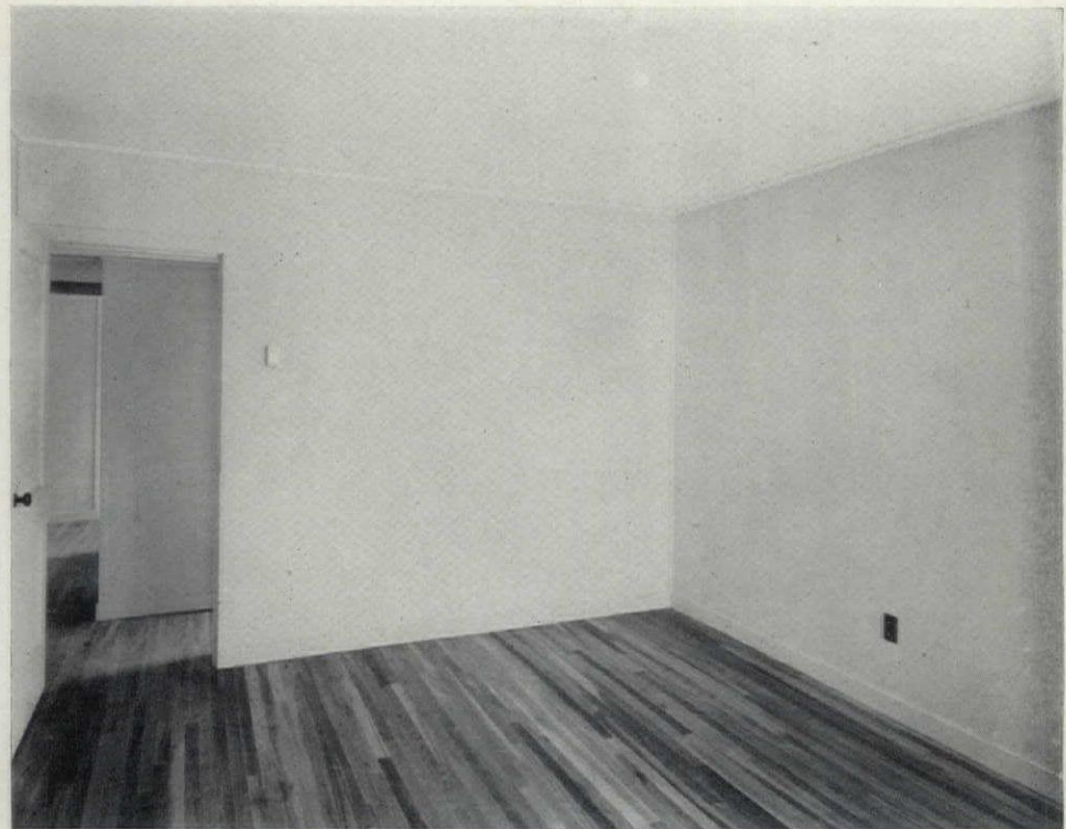
Interior of one of the units, showing dry-wall construc- tion.
