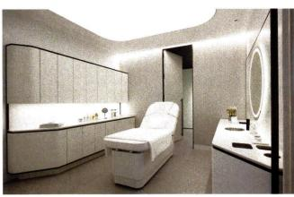
Inspired by flowing curtains, the pod is clad with rippled, interlocking MDF-backed fiberglass planks in a creamy, opalescent finish that appears as though glowing from within. For contrast, BHA and the fabrication team used bronze as trim along the edges of the freestanding structure, as well as for the hardware, carrying the metal's rich hue to the recycled-oak floor, existing radiators, and walnut ceiling slats.
