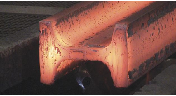
This beam blank is exiting the caster prior to reheating and rolling into a structural section.
