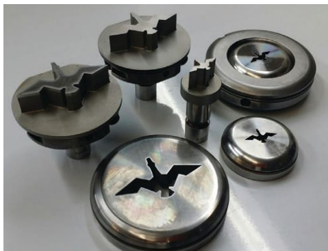
Customized cookie-cutter dies were manufactured as the shape of the holes in the acoustic ceiling throughout the Sports Center at the University of Oregon.
