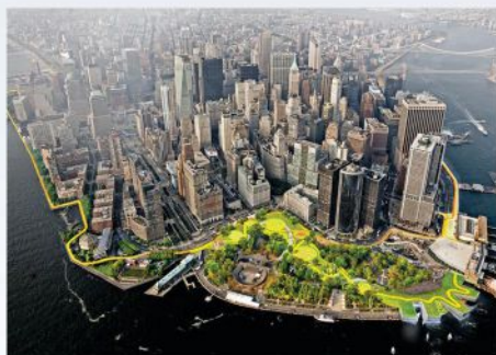
LafargeHolcim Awards Silver 2014 – $50,000. The Dryline (BIG U) addresses the vulnerability to coastal flooding with a protective ribbon in Southern Manhattan. Embankments that add green areas and spaces beneath elevated roadways are built out with pavilions for public use. New York, NY
