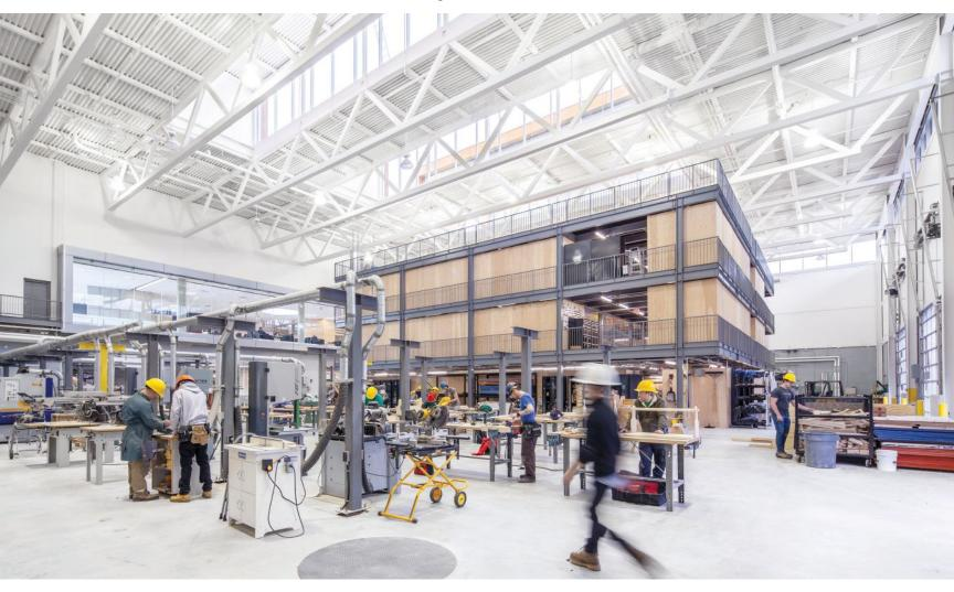
The technology center's Learning Factory (above) features a four-story teaching cube that provides a flexible framework for electrical and plumbing installations and a realistic simulation of actual site conditions.
