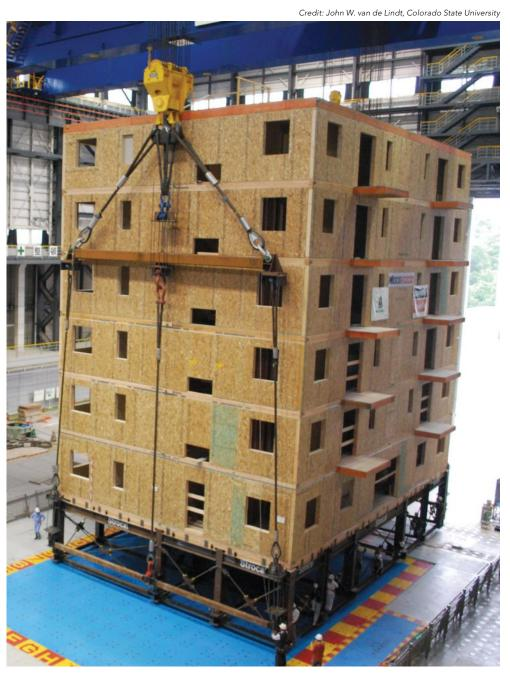
Subjected to three earthquakes on the world's largest shake table in Miki, Japan, this full-scale wood-frame apartment building performed excellently with little damage.
