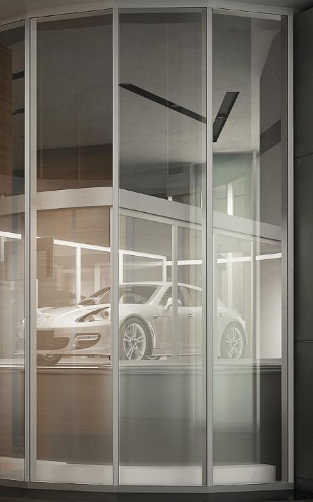
2 HOUR FIRE RESISTIVE GLASS INTERIOR/ELEVATOR ENCLOSURE WITH SUPERLITE II-XL 120 IN GPX CURTAIN WALL FRAMING
