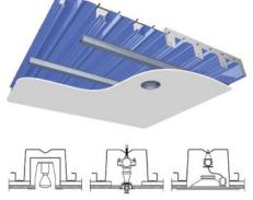
Composite concrete and steel floor systems gain their strength from the shape and height of the metal deck that receives the concrete. In some profiles, the underside spaces are large enough for small utilities to be run, such as lighting, sprinklers, or sound components.
