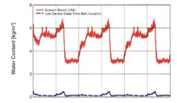
(Top) Water content in exterior sheathing with nonpermeable air barrier—Chicago (CZ5). (Left) Moisture content of exterior sheathing with permeable air barrier— Chicago(CZ5).
