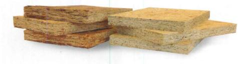
High-performance engineered wood panels show considerably less swelling from moisture absorption after a 24-hour water soak test, when compared to traditional OSB.
