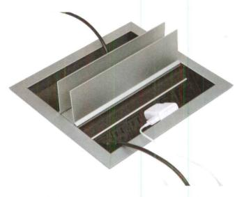
Dual-sided PCS54/2 sits beneath the surface for a clean look on any table. A thin, hinged lid cover opens to reveal two electrical outlets rated 15A/125VAC, one Category 5e data module and one dual input USB charger for charging mobile devices. Angled face provides optimal accessibility on both sides.
