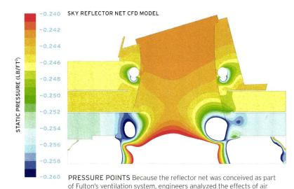
movement on the device, relying on computational fluid dynamics.
