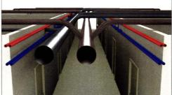
Hospital patient room hall interstitial space for all-air HVAC system (supply, return, and exhaust) vs. hospital patient room hall interstitial space for an active chilled beam application (supply duct, exhaust duct, chilled water piping)
