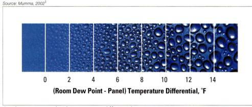
Condensate on panel with temperature differential
