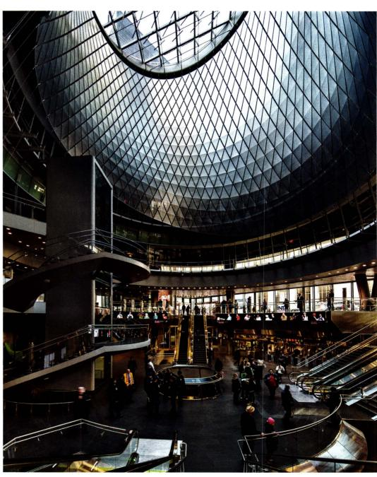
Created with James Carpenter, the oculus, with its perforated aluminum panels, draws daylight into the station.
