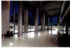
At Chabot College in Hayward, California, designers wanted to incorporate as much glass as possible to flood the interior with daylight and keep a connection to the outdoors. Electrochromic glass was used (clear on left and tinted on right) instead of mechanical shades or blinds in order to retain the view and keep the openness of the space.
