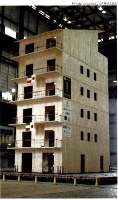
Seven-story CLT building being tested on the world's largest shake table in Miki, Japan
