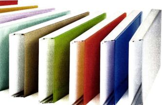
This insulated unitized daylighting system by CPI Daylighting comprises a double layer of translucent, quad-glazed, Nano-Cell polycarbonate panels (made up of 10% postindustrial content) held by recycled-aluminum framing. Features include long-span capability, bicolor and scalable performance options, and an easily removable and replaceable exterior skin.
