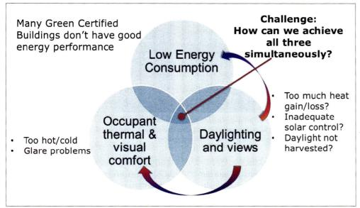
A pictorial representation of the challenge of green building design: how to optimize both energy efficiency and daylighting and views without compromising occupant comfort.
