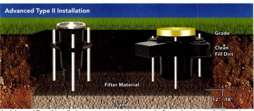
An Advanced Type II installation creates a trench between the fixture housings to facilitate the drainage of water away from the surface.
